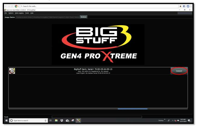
**Step 4.2** – Below, is the BCP default **Main Dashboard** window that opens after selecting **Connect** in Step 4.1. For this example, **Jim Jackson Serial 70-B3-D5-64-E0-15** is the Project running in the BCP software on the PC. For your application, **Your Name Serial 70-B3-D5-64-XX-XX** will be the Project running in the BCP software on the PC.
