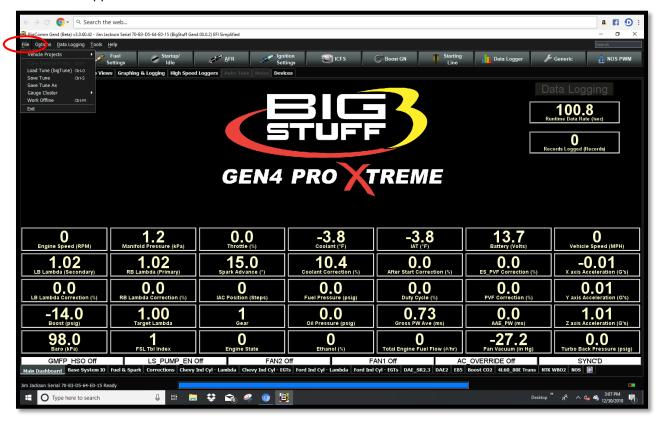
**Step 5.2** - Once **File** is selected in Step 5.1, a drop-down window will open. Once opened, highlight and left mouse click on **Save Tune As** as shown below.
